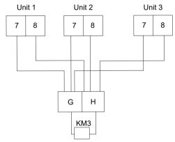
When one auxiliary electric heater serves more than one modules, its wiring terminals (7 and 8) are connected to terminals (G and H) for an AC contactor KM3.
