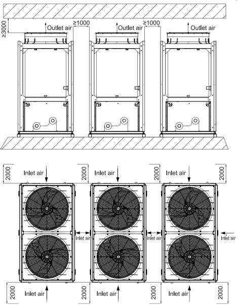
Note: the unit shall be equipped with shock-absorbing rubber pad (provided by the user), and then fixed on the ground or roof with bolts. The above figure is just for reference, not in actual scale.
