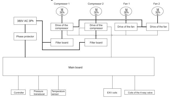
Note: bold lines indicate the main circuit and slim lines indicate the contorl circuit.
