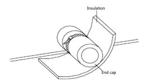
Insulation should be thickened at humid areas.
