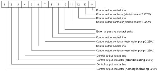
Note: the output control lines of the AC contactors for the running indicator, water pump 1, water pump 2, auxiliary electric heater 1, auxiliary electric heater 2 can be wired to the corresponding wiring board of all units, while those for the error indicator and external passive contact switch should be wired to the corresponding wiring board of all units.
