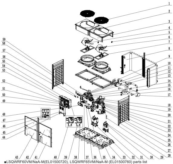
No. Name Quantity Rear Gril Coping Top Cover Axial Flow Fan Axial Flow Fan Nesting Brushless DC Motor Motor Support Sub-Assy Condenser Assy Temp Sensor Sleeving 4-way Valve Filte Magnet Coil Rear Grill 1
