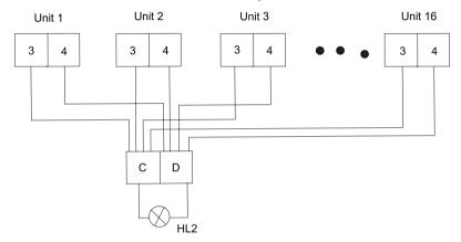
When it is required to display errors of several units, the wiring terminals (3, 4) of each unit should be wired to the wiring terminals HL2 (C, D) of the error indicator. (If it is required to display the error of each unit independently, then the error indicator of each unit should be wired independently to the corresponding error output wiring terminals (3,4) of each unit.
