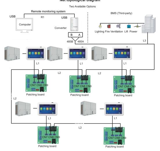
Note: the system as shown in the figure above consists of 1~16 single units depending on the actual demand of the project.
