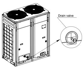
Drain valve for LSQWRF35VMP1/NhA-M
