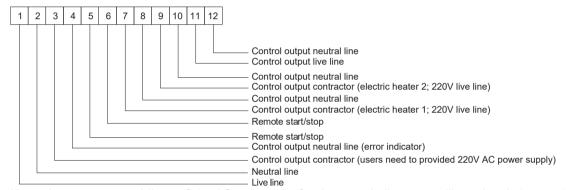
Note: the output control lines of the AC contactors for the error indicator, auxiliary electric heater 1, auxiliary electric heater 2 can be wired to the corresponding wiring board of all units, while those for the error indicator and dry contact switch should be wired to the corresponding wiring board of all units as shown in the figure below.
