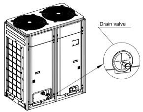
Drain valve for LSQWRF35VMP1/NhA-M
