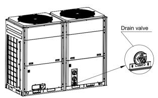
Drain valve for LSQWRF60VMP1/NhA-M
