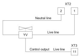
Example 2: If the project uses a 3-point floating type 2-way motorised ball valves, wiring will be conducted as described in the diagram below.
