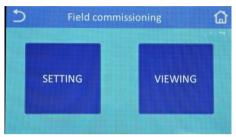
(5) Click the "Setting" key and turn to the second page of "FIELD SETTIGN", and then click "Water pump speed" to set the standby speed of the water pump.
