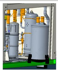
Loosen fixed screws and take out the vapor-liquid separator.
