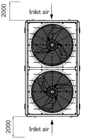
Note: the unit shall be equipped with shock-absorbing rubber pad (provided by the user), and then fixed on the ground or roof with bolts. The above figure is just for reference, not in actual scale.
