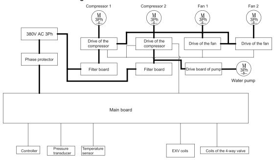
Note: Bold lines indicate the main circuit and slim lines indicate the control circuit.
