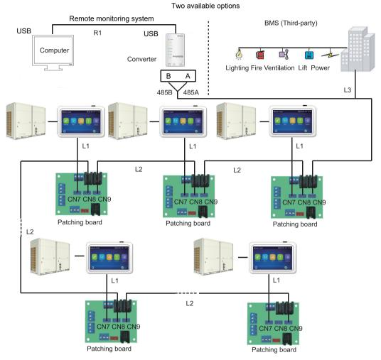
Note: the system as shown in the figure above consists of 1 to 3 single units depending on the actual demand of the project.
