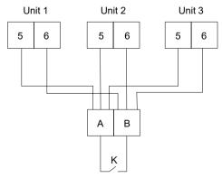
When external passive contact switch is available for multiple units, the wiring terminals (5 and 6) of each unit should be wired to the terminals (A and B) for a dry contact switch.
