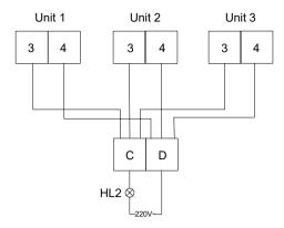
When it is required to display errors of several units, the wiring terminals (3 and 4) of each unit should be wired to the wiring terminals (C and D) of the error indicator HL2. (If it is required to display the error of each unit independently, then the error indicator of each unit should be wired independently to the corresponding error output wiring terminals (3 and 4) of each unit.
