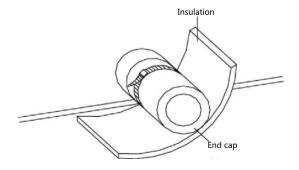
Insulation should be thickened at humid areas.
