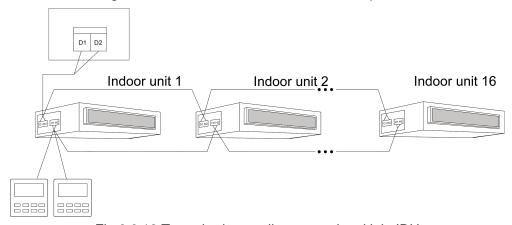
Fig.3.9.12 Two wired controllers control multiple IDU
