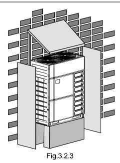
(2) Anti-monsoon installation requirements for unit connecting exhaust duct:
