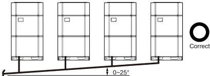
Piping between modules is under the module pipe connector and increases upwards with an angle of 0° to 25°.
