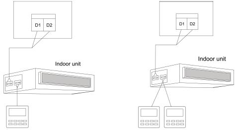
Fig.3.9.9 One wired controller controls one IDU Fig.3.9.10 Two wired controllers control one IDU
