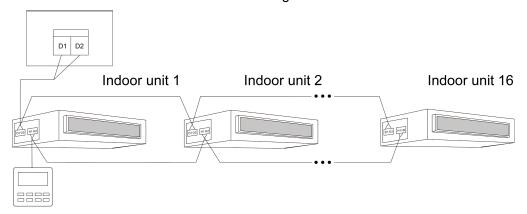
Fig.3.9.11 One wired controller control multiple IDU
