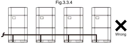
Piping between modules is above the module pipe connector.
