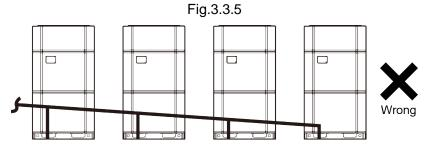
Piping between modules is above the module pipe connector.
