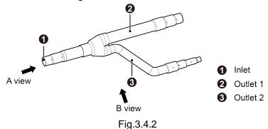
2) Manifold has several pipe sections with different pipe size, which facilitates to match with various copper pipes. Use pipe cutter to cut in the middle of the pipe section with different pipe size. See the Fig. 3.4.3 as below.
