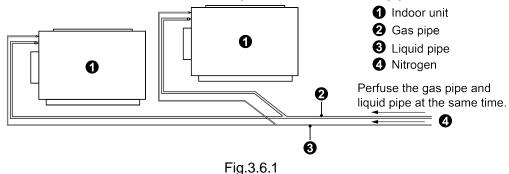
**NOTE**: All welding points can't be heat-insulated and wrapped until the air tightness test is completed.
