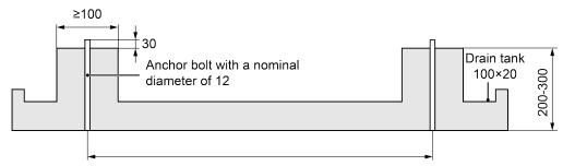
The distance is determined based on the actual size of the unit
