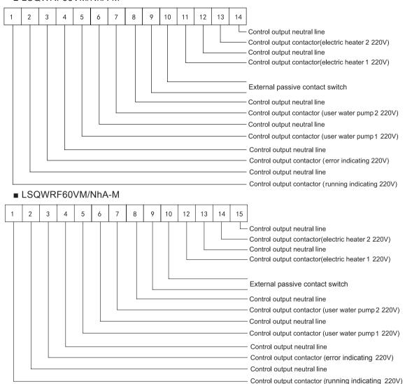
Note: the output control lines of the AC contactors for the running indicator, water pump 1, water pump 2, auxiliary electric heater 1, auxiliary electric heater 2 can be wired to the corresponding wiring board of any one unit, while those for the error indicator and external passive contact switch should be wired to the corresponding wiring board of all units as shown in the figure below.
