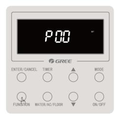
Step 4: Hold on pressing "FUNCTION" button for 5s and then POO will be displayed;
