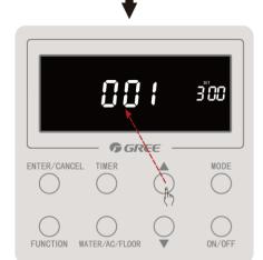
Step 7: Press " $\blacktriangle$ " or " $\blacktriangledown$ " button to select the sequence (1^3) of hydro box for setting; Note: If selection is not needed, next step can be entered;
