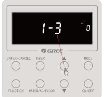
Step 9: Press "▲" or "▼" button to select the sequence(1~6) of shunt valve for setting; Note: If selection is not needed, next step can be entered;
