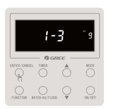
Step 12: Press "ENTER/CANCEL" button to confirm the setting of current shunt valve and indoor unit; Note: 1. If you need to set the shunt valve and indoor unit of other hydro box, please repeat step 6 to step 12 (for one wired controller controlling several units or several wired controllers controlling several units) or repeat step 8 to step 12 (for one wired controller controlling one unit);
