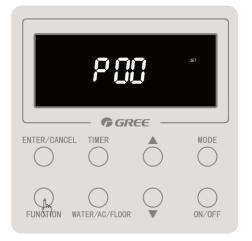
Step 4: Hold on pressing "FUNCTION" button for 5s and then POO will be displayed;
