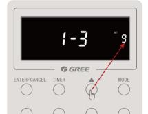
Step 11: Press "▲" or "▼" button to select the indoor unit(project no. 1^255) for setting; Note: If selection is not needed, next step can be entered:
