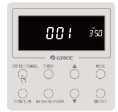
Step 10: Press "ENTER/CANCEL" button to confirm the water tank capacity setting of current hydro box;
