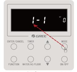
Step 6: Press "MODE" button to enter hydro box selection setting;
