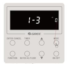
Step 10: Press "MODE" button to enter indoor unit selection setting
