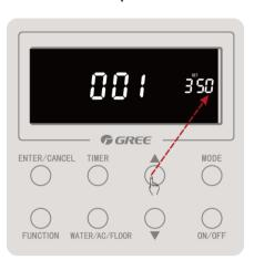
Step 9: Press " $\blacktriangle$ " or " $\blacktriangledown$ " button to set water tank capacity;
